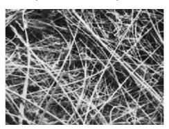
**MS**<sup>®</sup> Glass fiber filters are manufactured from 100% borosilicate glass. These depth filters combine fast flow rate with high loading capacity and retention of fine particulates. The small diameter fibers give glass fiber filter media superior efficiency and dirt holding as compared to cellulose and synthetic media.
