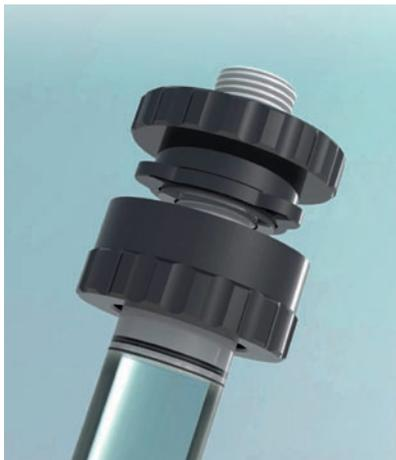
No more than a quarter turn is needed to seal the column. Piston height adjustment is done by turning the locked “Quick-Lock” fitting.
