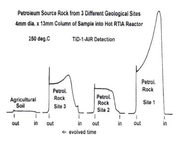
column inside 6mm OD x 4mm ID glass tube tube inserted and sealed into reactor so incoming Air flowed through tube ID and the samples sample tubes inserted/removed as indicated peak in signals followed by decay indicates constituent being volatilized and removed - steady signal plateau indicates constituent vapor pressure, but no volatilization/removal.
