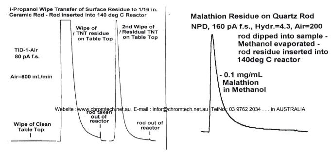
dried TNT residue on a table top wiped with an iso-propanol pad and transferred to ceramic rod.
