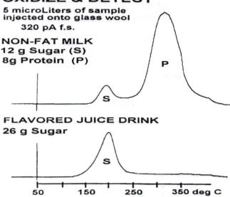
crushed rock/sositionsebjirpatekedtimto-beinologomometariation of the 78787134 technique AliaTID-1 detector mounted onto a GC - 2 inch long 6mm OD x 4mm ID open end glass tube packed with glass wool located inside GC oven and connected to detector inlet - sample pump at detector exit pulled Air through the system - liquid samples injected onto column oven temperature programmed to provide profile of oxidation product signals vs. temperature.
