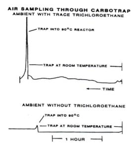
RTIA/TID-1. 1 L/min ambient Air - 1 hour through unheated trap, then trap into 90°C reactor.
