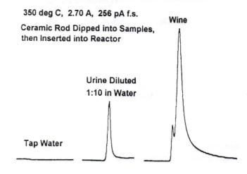
water based liquid samples - ceramic sample rod moist with both water and residual organic material when inserted into the reactor - signals mostly due to oxidation products of the organics.
