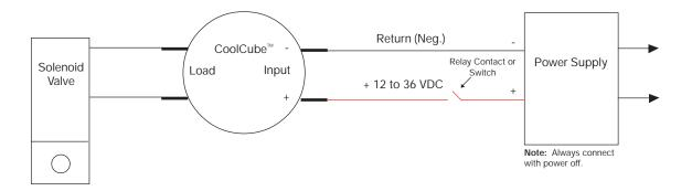
1. Using an AMP\*, Molex or similar connectors, connect the CoolCube<sup>™</sup> to the DC power supply.
