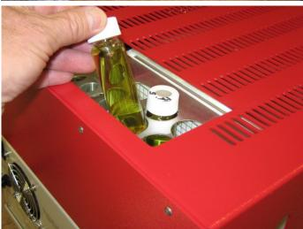
The GC includes SRI's Flame Ionization Detector (FID) which is able to measure the cannabinoid molecules based on its ability to detect the combustion of hydrocarbon molecules.
