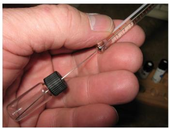
With 2-3ul of liquid in the syringe, hold the needle vertically or at least slanted upwards so any air bubbles will rise towards the needle.
