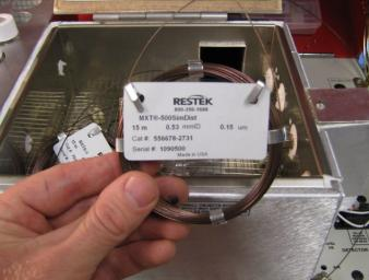
The residual solvent analysis can also be performed on the MXT-500 column that comes standard with the Potency GC, but the separation of volatile hydrocarbons will not be as good. For the best separation of terpene molecules, a 30 meter MXT-Wax is recommended but solvent separation will not be as good, and buying the column will be more expensive. As with all GC analysis, the operator must decide what compounds are most important to detect and select the proper column accordingly.
