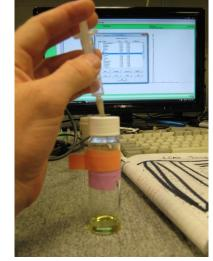
With the syringe plunger still at the 1mL mark, place the needle up against the septum of the injection port (but not poking through it yet). Press the Start Run button or press the spacebar on the keyboard.
