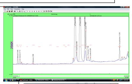
The Results screen will display the area counts of all peaks detected and identified with retention windows.
