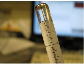
With air bubbles removed, push the plunger to the 1ul mark. It is important to be as precise as possible. Wipe the needle with your fingers or a tissue to remove any liquid from the outside of the needle.
