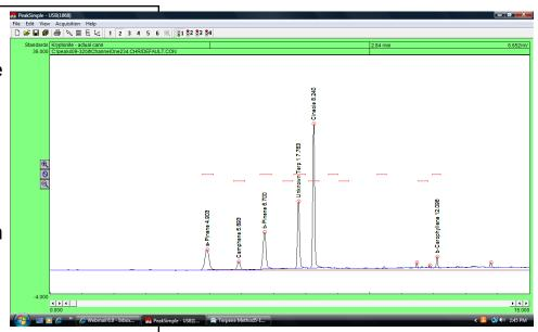
The Results screen will display the area counts of all peaks detected and identified with retention windows.
