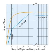
Figure 2 Sample mass (observed peak area) vs. volume of sample dispensed from the syringe, in units of loop volumes, injected onto the column from our dual mode injector such
