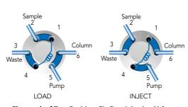
Flow path of Two-Position, Six-Port Injection Valve
