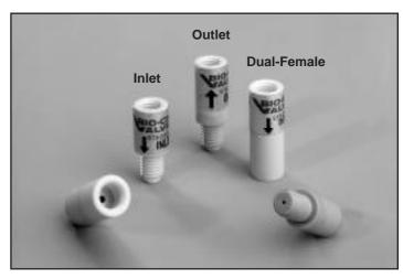
The *Bio-Chek™* self-sealing in-line check valves feature an inert flow path, no metal components and zero maintenance in high-purity, low-pressure applications.
