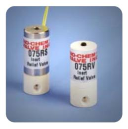
The 075RV / 075RS relief valve series is ideally suited for use with aggressive and high-purity fluids. Wetted parts consist of the PPS (Ryton) valve body and the Chemraz® diaphragm. Custom body and diaphragm configurations are available from a broad menu of engineered plastics and elastomers, including Teflon®. The unique Bio-Chem Valve diaphragm retention design ensures the most reliable performance and longest life available.
