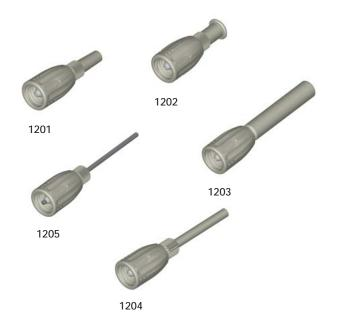
These adaptors can replace the Omnifit cap on any 'Omnifit Cap' connector or valve to give either quick push-on connections for softwall tubing or luer connections. Cap-to-luer adaptors are available with male or female luer connections. Cap-to-pipe adaptors are available in Tefzel® or stainless steel to accept softwall tubing with the following internal diameters: 1/16", 1/8" and 1/4".
