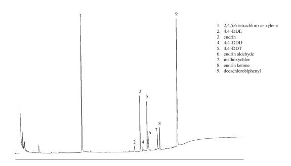
30m, 0.53mm ID, 0.42µm Rtx®-CLPesticides2 (cat.# 11340). **On-column conc.:** 50ppb; **Oven temp.:** 120°C (hold 1 min.) to 300°C @ 9°C/min. (hold 10 min.); **Inj./det. temp.:** 250°C/300°C; **Purge:** on 0.75 min.; **Carrier gas:** helium, 33cm/sec.
