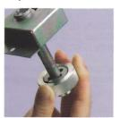
Screw the rethreading tool completely onto the injection port in a clockwise direction
