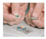
Dislodge ferrules or remove silica deposits with the Jet Reamer/Ferrule Remover.
