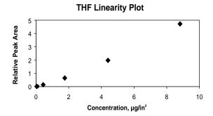
Tested over an approximate concentration range of 0– $10 \mu g/in^2$  for each component.  $R^2 = 0.992$  (THF), 0.985 (benzene), and 0.994 (styrene).
