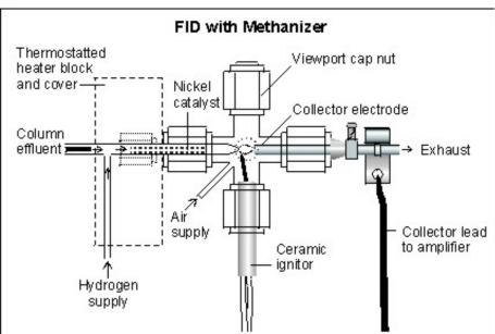
The special Methanizer FID detector assembly operates like the regular SRI <u>FID detector</u>, except that the FID temperature must be set to 380°C. Due to the chemical relationship between nickel and sulfur, the Methanizer can be poisoned by large quantities of sulfur gas.
