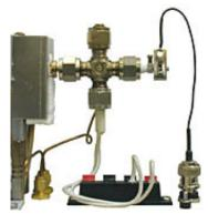
The Methanizer option enables the Flame Ionization Detector to detect low levels of CO and CO<sub>2</sub>. It is installed as the removable jet in a special FID detector assembly. The Methanizer is packed with a nickel catalyst powder. During analysis, the Methanizer is heated to 380°C with the FID detector body. When the column effluent mixes with the FID hydrogen supply and passes through the Methanizer, CO and CO<sub>2</sub> are converted to methane.
