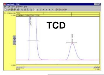
This chromatogram is from a direct injection of 0.5mL of human breath. The longer we hold our breath, the higher the CO<sub>2</sub> content. This was the result of a class experiment called "Waiting to Exhale," which is included in the manual. It is a contest to see who can blow the most CO<sub>2</sub>. Participants merely exhale into a 3mL syringe, then inject 0.5mL into the on-column injector of an Educational TCD GC.
