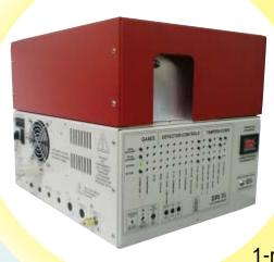
CCD - Detects Hydrocarbons & Hydrogen
