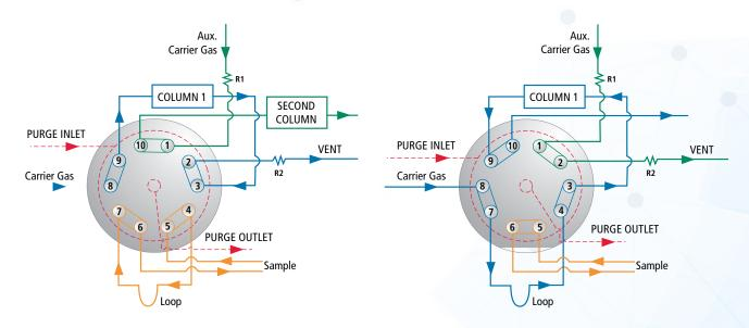
Figure 9: Gas sampling and backflush to vent
