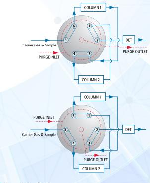
Figure 7: Foreflushing
