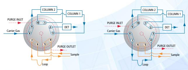
Figure 10: Gas sampling and sequence reverse
