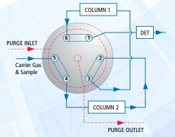
Figure 4: Backflush and sequence reverse
