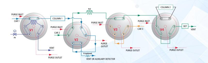
Figure 13: **Configuration variation**Here V4 is added to allow column 2 by-pass.
