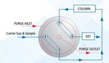
Figure 2: Backflush column to detector
