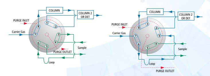
Figure 8: Gas sampling and backflush to detector
