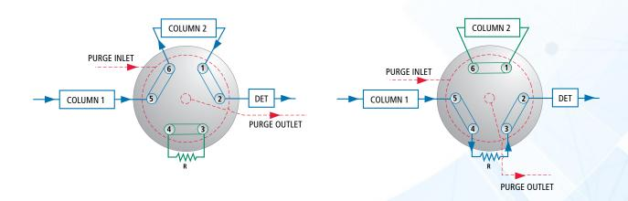
Figure 5: Column isolation - method 1
