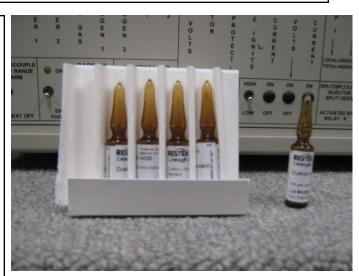
Break the glass ampoule and transfer the contents into a 2ml septum vial (Restek #21154 and #24495). Restek provides one free vial with each standard.
