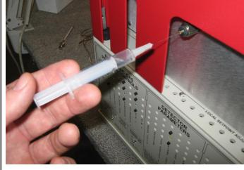
The picture at right shows a terpene sample vial filled to the neck with extraction solvent and ready to be injected for cannabis potency analysis. See the PeakSimple tutorial describing the process for Medical Cannabis Potency Testing.
