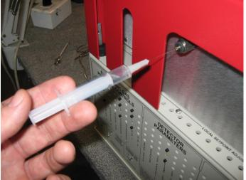
The picture at right shows a terpene sample vial filled to the neck with extraction solvent and ready to be injected for cannabis potency analysis. See the PeakSimple tutorial describing the process for Medical Cannabis Potency Testing.
