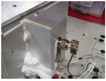
The cannabinoid molecules, Δ9-THC, CBD, and CBN (and for more advanced operators, CBC, Δ8-THC, and CBG) are separated by a 15-meter metal capillary column which is heated in the column oven.
