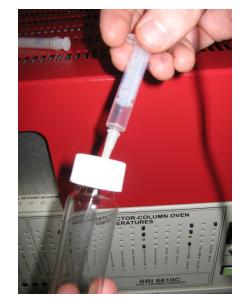
Inject the contents of the syringe into the injection port and start the run as shown previously.
