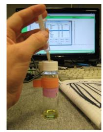
With the syringe plunger still at the 1mL mark, place the needle up against the septum of the injection port (but not poking through it yet). Press the Start Run button or press the spacebar on the keyboard.
