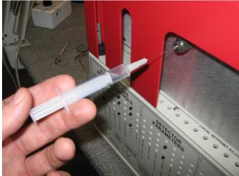
Insert the syringe all the way through the septum as far as it will go. Immediately depress the plunger and quickly withdraw the syringe.
