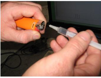
To identify gasoline and its constituents that remain after evaporation (BTEX) obtain some gasoline and place it into an airtight vial. Using the 3 mL syringe, suck out 1 mL of headspace gas from the top of the vial.
