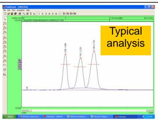
potency can be tested on the same GC platform. Alternate detectors such as FID (Flame Ionization Detector) may be substituted on request.
