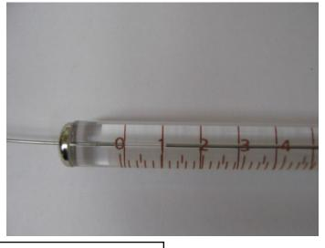
Pull the plunger back to the 3ul mark and note the amount of liquid. It should be 1.6-1.8ul because the needle also contains .6-8ul and this adds to the 1ul you measured with the plunger.
