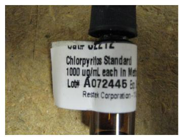
Deposit 1ul of the CPP standard on a clean cotton wad in the tube.
