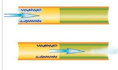
a) Sample introduction: liquid film of solvent and sample are deposited in the first length of capillary.
