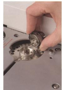
The new way: with the EZ Twist Top™ Injection Port, the gas lines are under the GC cover and are not disturbed during maintenance.
