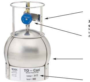
2 or 3 Port high quality valve Metal-to-metal seal, 2/3 turn with stainless steel diaphragm.
