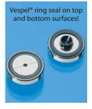
In Agilent split/splitless injection ports, it can be difficult to make and maintain a good seal with a conventional metal inlet disk. The metal-to-metal seal dictates that you apply considerable torque to the reducing nut, and, based on our testing, this does not ensure a leak-tight seal. Over the course of oven temperature cycling, metal seals are prone to leaks, which ultimately can degrade the capillary column and cause other analytical difficulties.
