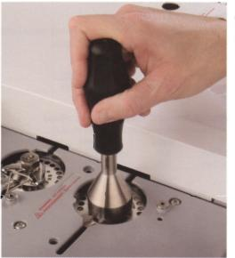
Simply slip the Weldment Removal Tool over the weldment, then twist and remove the weldment. For speed and efficiency, the weldment stays secured in the Weldment Removal Tool until you reattach it.
