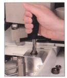
Turn counterclockwise to loosen liner cap.
