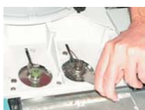
Use the larger end to tighten the split/splitless weldment nut.
