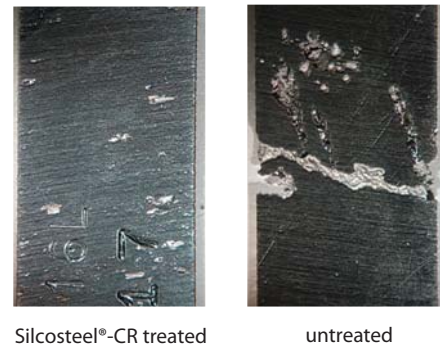
Figure 5 Silcosteel®-CR treated 316L stainless steel shows no crevice corrosion and only slight pitting corrosion after 72-hour exposure to ferric chloride; untreated steel exhibits severe crevice corrosion.
