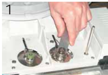
Use the smaller end to remove the septum nut.
