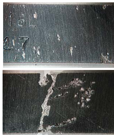
Figure 1 Silcosteel®-CR treated 316L stainless steel coupons show no crevice corrosion and only slight pitting corrosion (top), while bare 316L stainless steel coupons exhibit severe crevice corrosion (bottom).
