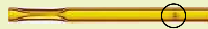
Figure 1 The drilled hole in a Uniliner® injection port liner makes direct injection possible with EPC systems by equalizing pressure in the injection port.
