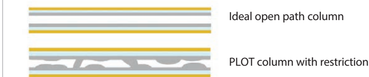
Figure 2: Inconsistent coating thicknesses result in restrictions that cause significant variation in flow.
