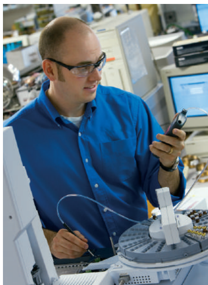
Checking for leaks, using a Restek® electronic leak detector, is an easy way to protect your instrument and column from damage.
