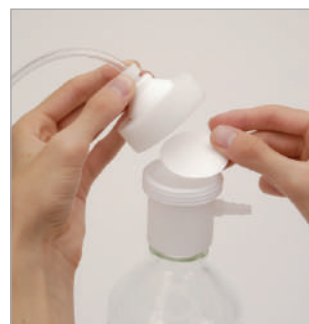
Place membrane filter on top of grid.
