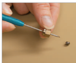
Dislodge a stuck ferrule quickly and easily—without scoring the fitting.
