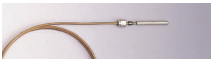
Adaptor kit centers the packed column in the injection port, so the syringe will not scrape the sides of the column.
