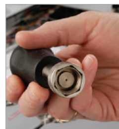
Septum nut remains in tool until reinstalled.
